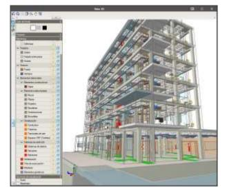
The remaining IFC files are those corresponding to the building services of the building, such as lighting thermal loads, electricity, fire safety, etc.
